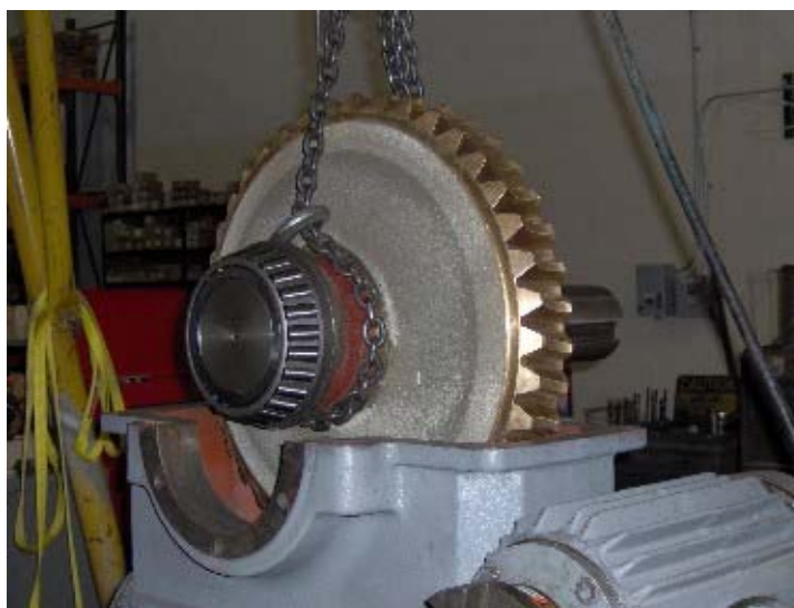
Replacement Worm Gear installed
